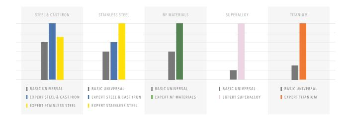
**The** tool matrix for our BCU1 Series compares the performance of individual milling cutters within the series. The values clearly show the performance in relation to the respective property in order to help you choose the right tool for every requirement.
